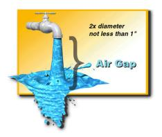
The best method of preventing backflow is an air gap which either eliminates a cross-connection or provides a barrier to backflow. If an air gap is not practical, a mechanical backflow preventer, which provides a physical
